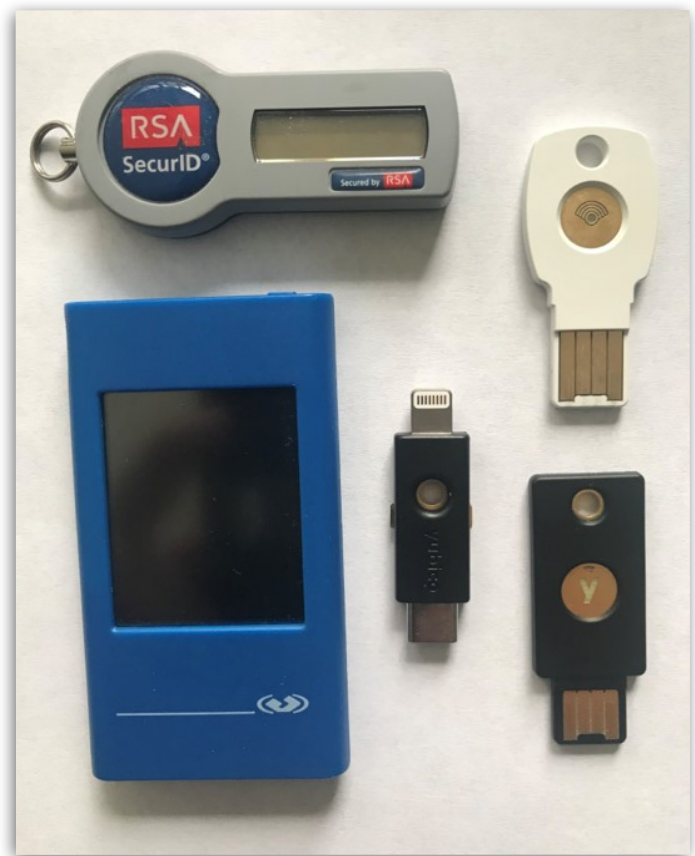
Various hardware keys used for MFA, including the latest FIDO-support keys along the right side and RSA's latest SecurID. (credit: D.Strom)
